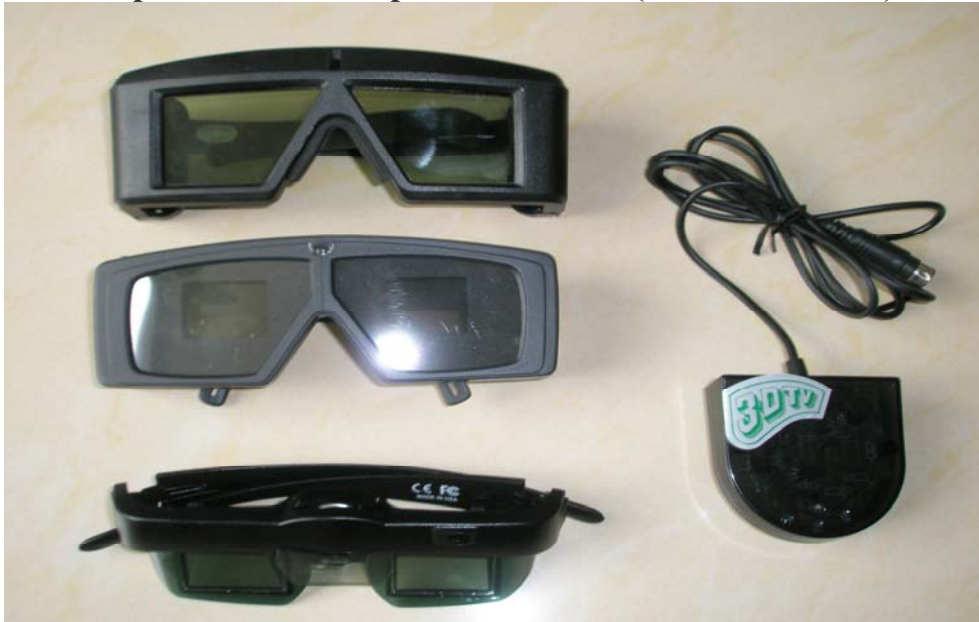
Fig 3 Universal Transmitter introduced by 3DTV Corp in 2008 with 3 of the many kinds of wireless LCD shutter glasses compatible with it.
